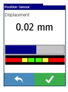
Easily position the Sensor using the Numeric Displacement readout and associated bar graph indictor
