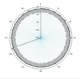
Radial plots show the overall shape of the profile. Overlay and align previous profiles to determine wear rates.
