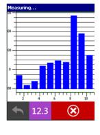
Live measurements can be displayed as a digital value or as a Shape Plot of the profile.
